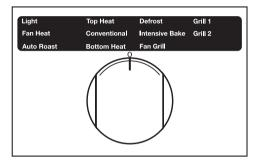
The function selector can be turned clockwise or anti-clockwise
